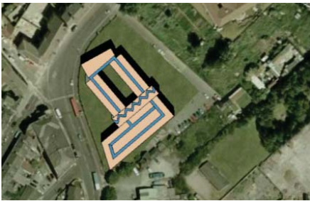
Early massing studies to determine best orientation and strategies for natural ventilation
